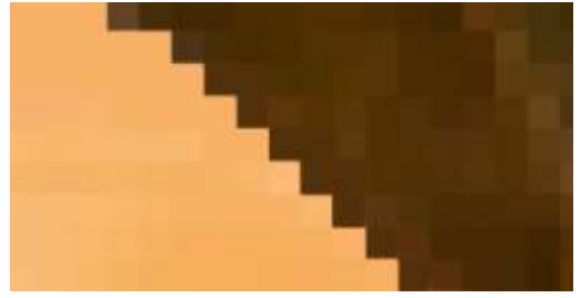
A camera sensor sees the world in a mosaic of small squares, unnatural jagged edges (sawtooth) are created on diagonals
